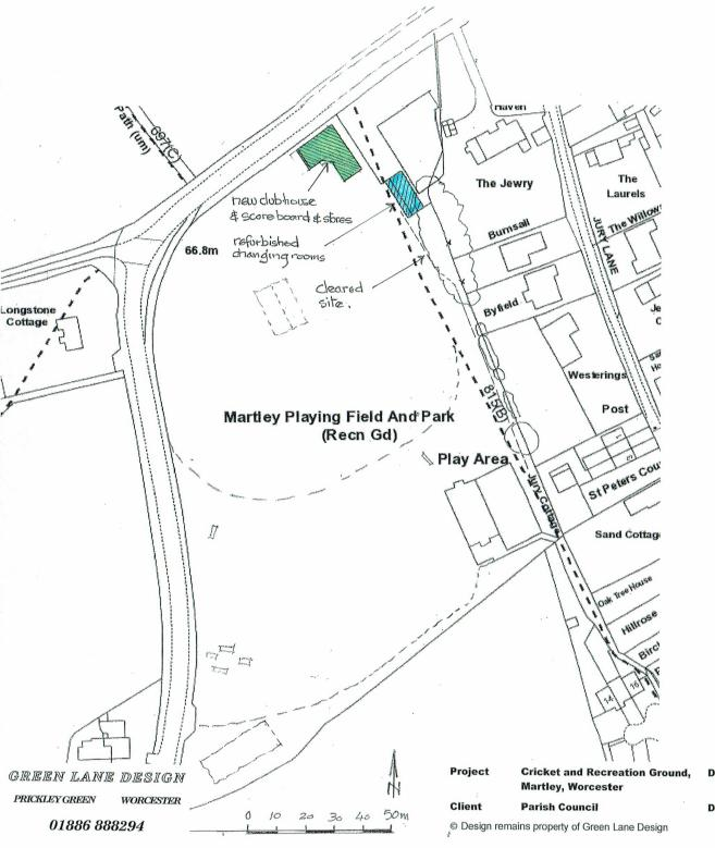
Option Two – refurbishment of existing pavilion and construction of additional service requirements – using alternative site by road.
